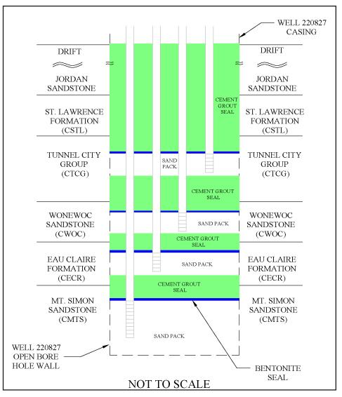
This schematic diagram depicts four new monitoring wells (referred to collectively as a well nest) located on the site of the now-sealed RPU Well No. 16 in Rochester. The well nest will be used to collect data about water quality and water levels' stability in four aquifers. **Graphic Credit:** Rochester Public Utilities
